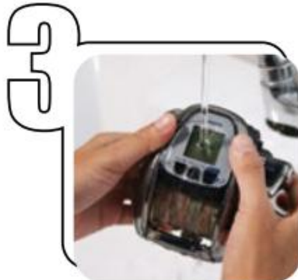
3 Quick run through of low pressure water on screen (not more than 3 seconds)
