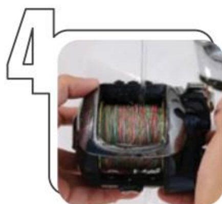
4 Rinse the spool area for removal of remaining salt
