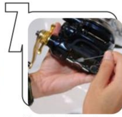
7 Use a tube brush to brush small accessible area (Reel seat, Line guide area) TO ENSURE removal of remaining salt
