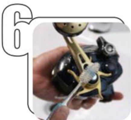
6 Use a toothbrush to brush the handle shank and handle knob area
