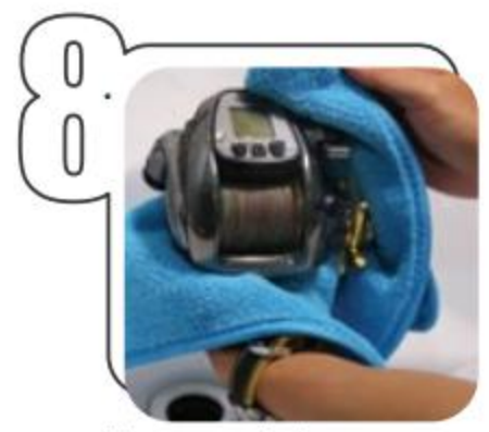
8 Use a wet cloth to wipe down the whole reel to ensure remaining salt and bait is removed
